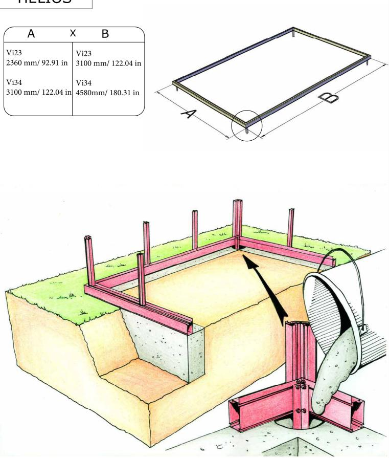
Note: While the foundation dimensions are provided above we reccomend that you layout the actual greenhouse frame before contruction of the foundation. This will eliminate any possible inconsistencies. Note: Do not fill in corners until the frame is full assebled. You may need to make small adjustements during assembly.
